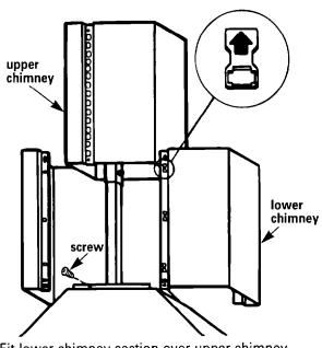
Fit lower chimney section over upper chimney section. Check for proper position. Then secure upper and lower chimney sections to support system frame with four screws.
